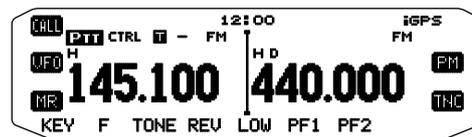
**Note:** When accessing a repeater that requires a 1750 Hz tone, you do not need to activate the Tone function. Simply press the key assigned to the 1750 Hz tone (Menu 906 ~ 911) to transmit the tone.
