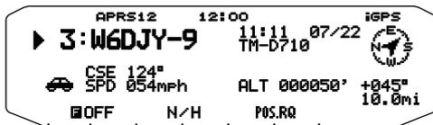
To change the speed/distance and/or temperature settings of the units, access Menu 626 (DISPLAY UNIT 1 - SPEED, DISTANCE) and/or Menu 626 (DISPLAY UNIT 1 -TEMPERATURE)
