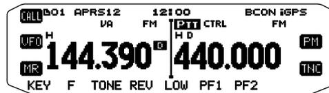
[RX ONLY]: A tone frequency is not added to the transmitted packet. "VAR" appears above the displayed frequency.
