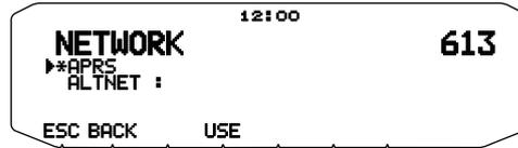
Set APRS data communications UNPROTOCOL. UNPROTOCOL is the method in which packet data is transmitted without other stations or making a connection.
