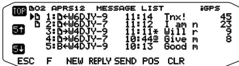
After entering a message on the message display, pressing the Tuning Control will cause it to transmit every minute.
