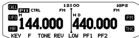
**Note:** When the transceiver overheats because of ambient high temperature or continuous transmission, the protective circuit may function to lower transmit output power.
