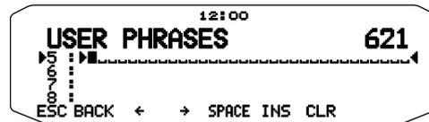
This function (clipboard image) allows you to paste phrases into the APRS message compilation mode. You can create up to 8 phrases each of which can consist of up to 32 characters.
