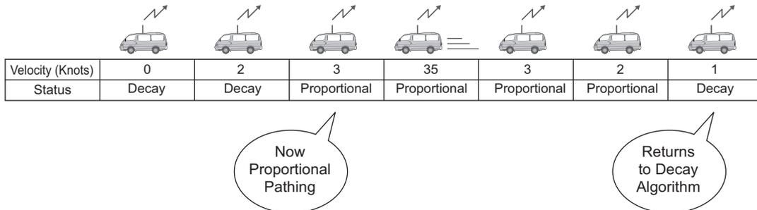
**Figure 6-3 Switching between Decay Algorithm and Proportional Pathing (when Stopped = 1 (knot); Moving = 3 (knots))**
