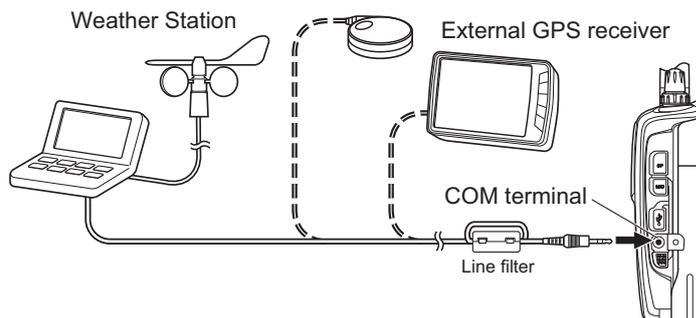
Figure 4-2 Connection Example of GPS Receiver
