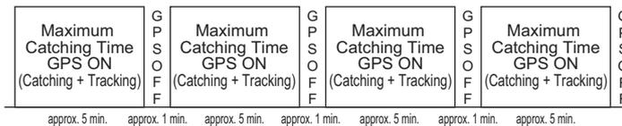
Figure 4-15 GPS Unit Behavior if 1 min is Selected
