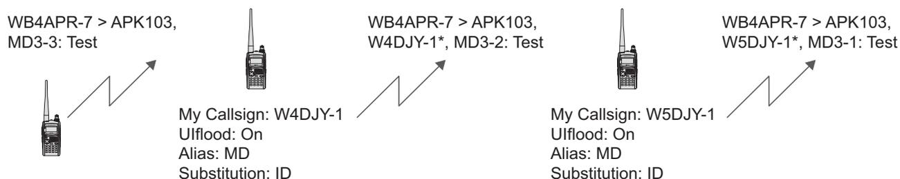
Figure 7-6 Using UIFLOOD
