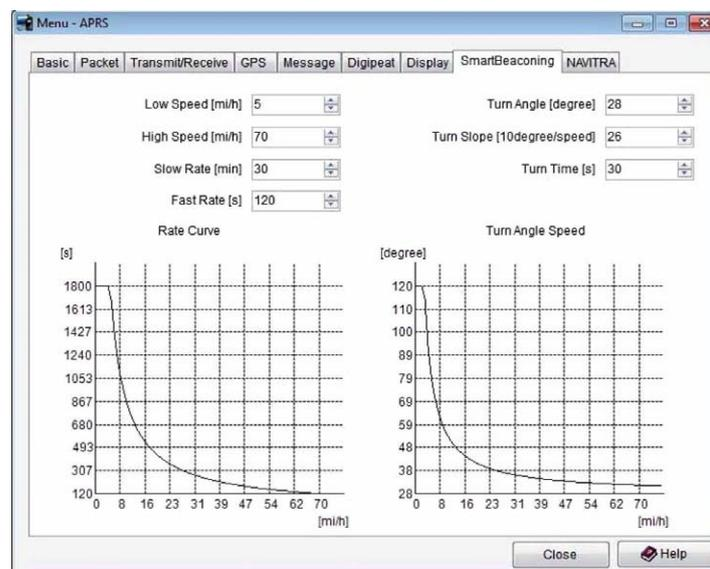
Figure 8-11 Graphs of SmartBeaconing
