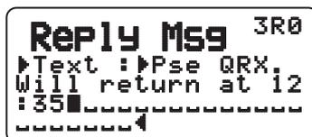
Figure 6-8 Automatic Reply Message Configuration Screen
