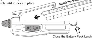
on the bottom of the radio, then slide the battery downward and out from the radio while tilting the Belt Clip out of the way.
